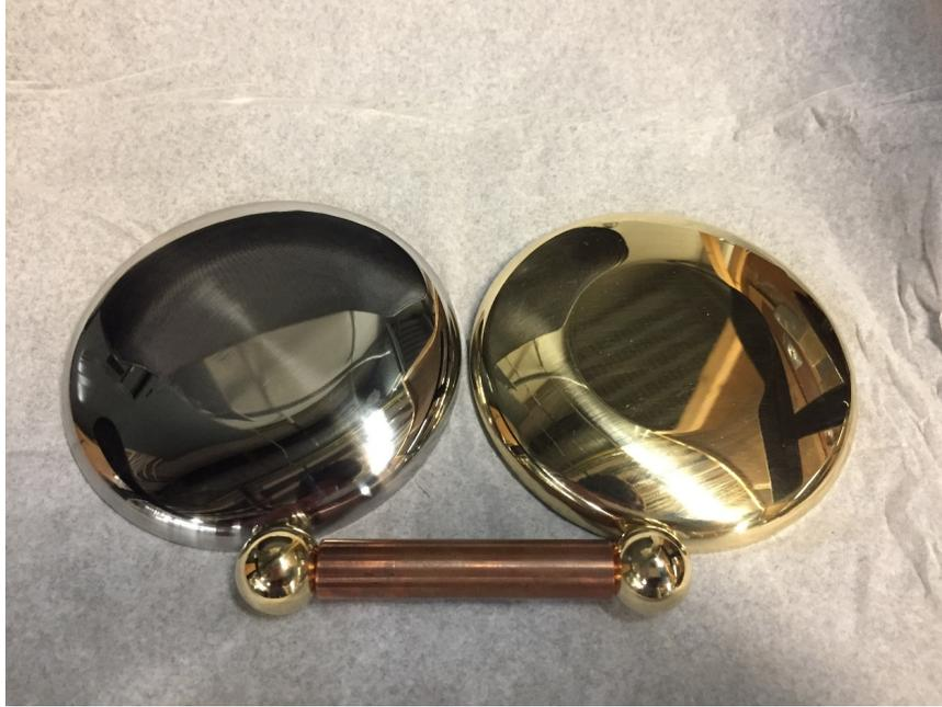
Figure 3.1. Brass and stainless steel Brass electrodes and brass spherical electrodes used in breakdown experiments.
