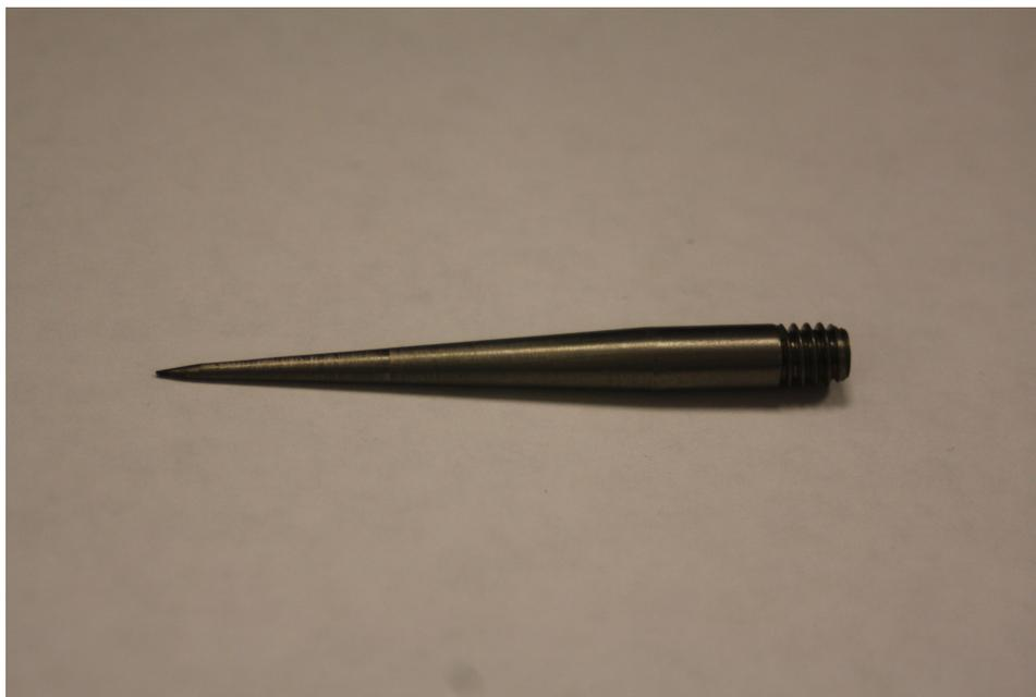
Figure 3.4. Machined tungsten needle used in initial DC and RF corona experiments.
