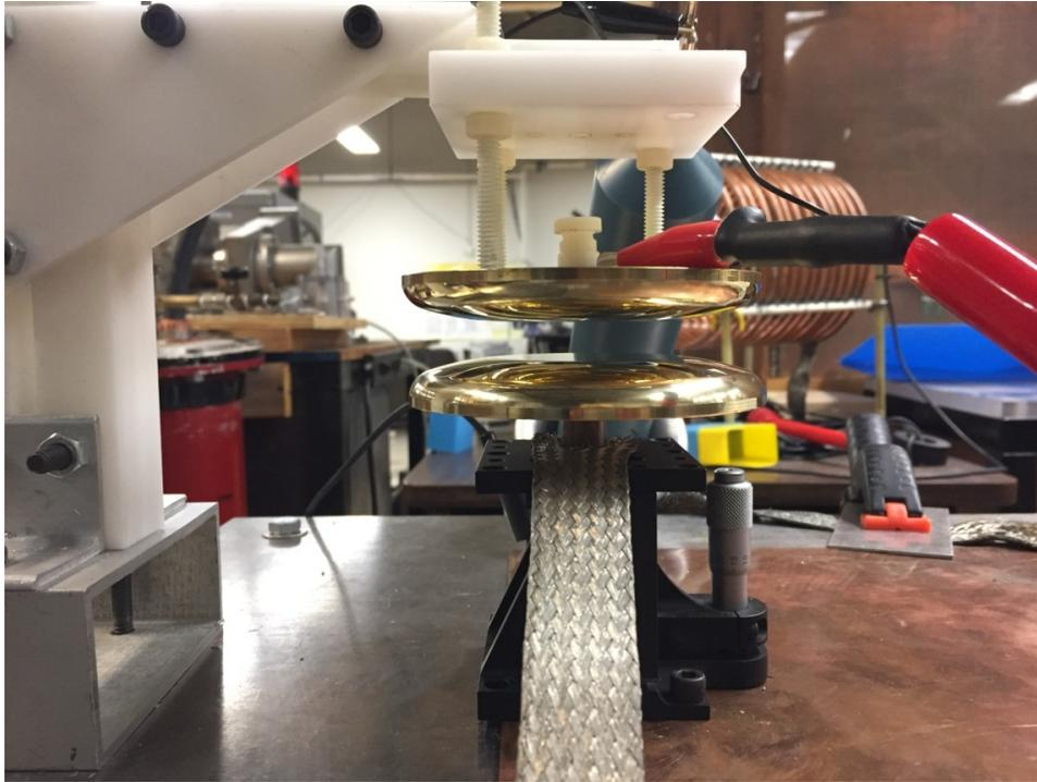
Figure 3.7. Gap setup for DC breakdown. A high potential tester and a commercial high voltage probe are connected to the top electrode while the bottom electrode is connected to ground. The electrode configuration shown is two brass Bruce profile electrodes separated by a 1 cm gap [4].
