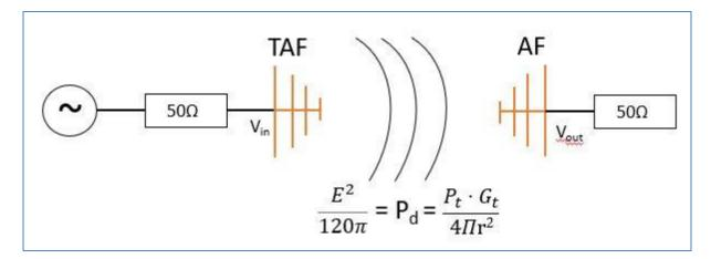
The antenna factor, AF, describes the capability of an antenna to convert its exposure to an RF E-field into a voltage on the output terminated with 50 ohms. Therefore we can write for the antenna factor
